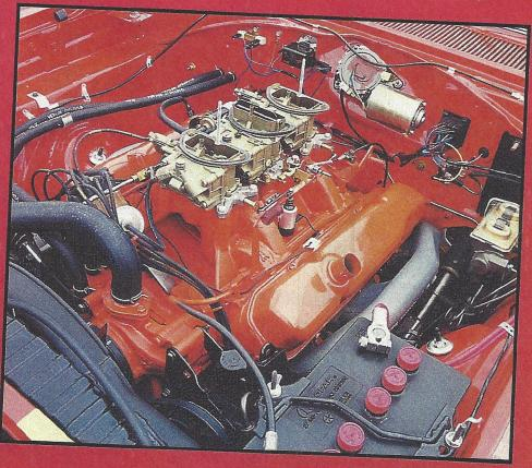
prove this quickly. All the wires are correctly coded, tagged, and every nut and bolt under there is phosphated, cadmium plated, or powder coated. Even the seat frames are powder coated!
