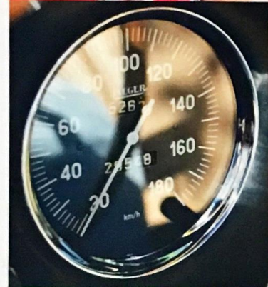
Apollo Speedo, registering kilometres per hour, but calibrated in mph
